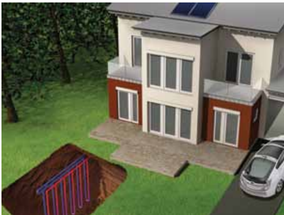
Vertical Ground Loop System
