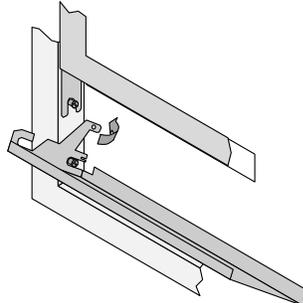
Bend the tab outward on both sides. This is the end-stop for the lower grill, it allows the grill to swing forward.
