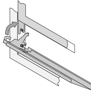
Swing the grill upwards to engage the upper slot. The grill fits inside the tabs for the barrier screen. You will need to lift the grill slightly to get it over the bushing. Once in place the grill is held in place by gravity.
