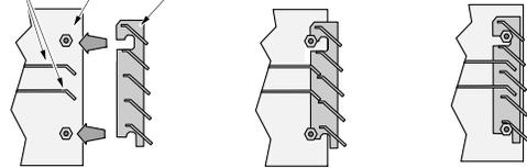
Position the grill so the slots on the grill align with the mounting studs.
